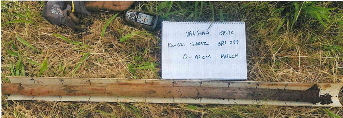
Soil core with coding, GPS reference, date etc
