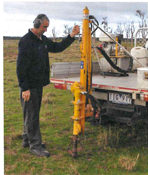
Soil sampling with hydraulic soil corer
